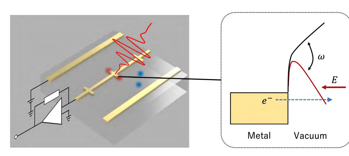
The intense optical field of infrared ultrashort pulses can control electron wave packets on the attosecond scale. We are developing a detector that can catch up with optical frequencies beyond 100 THz in combination with the field enhancement properties exhibited by metallic nanostructures.
