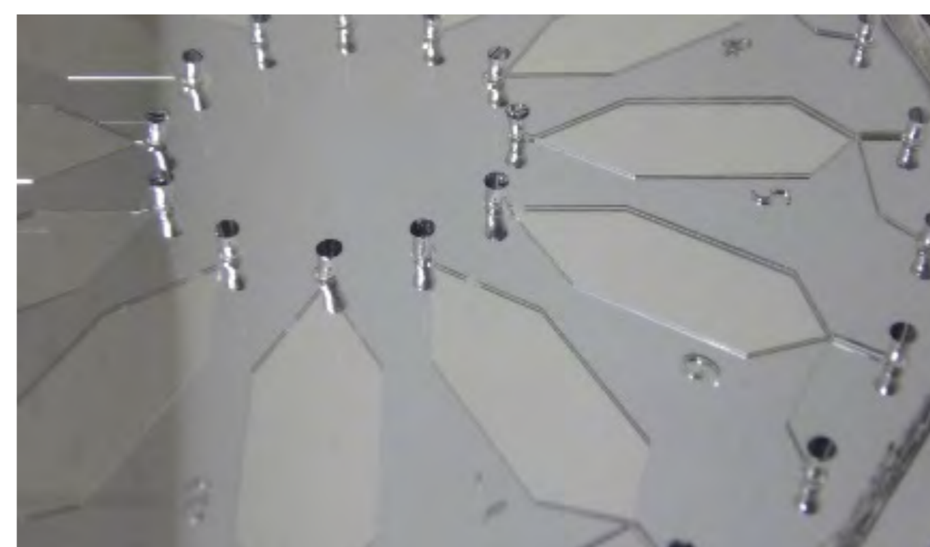
Microfluidic device for DNA purification
