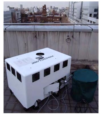
■ Wind velocity observation with a Doppler lidar
