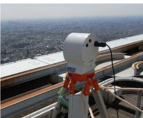
■ Estimation of heat fluxes using Scintillometer
