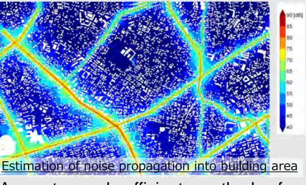
Accurate and efficient methods for creating environmental noise maps that are effective for environmental management are examined for noise source strength and noise propagation in build-up area. For source model, we propose a usage of aerial photographs and machine learning.
