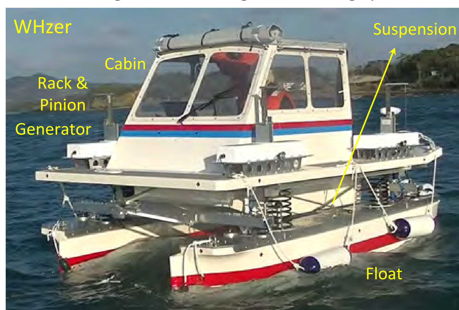
Wave Harmonizer (Yuya Bay; off Hiratsuka) Motion-controlled ship with wave energy harvester
