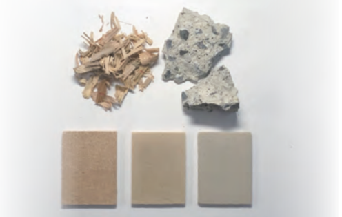
The recycled concrete with wood and concrete wastes. More concrete was used towards right.
