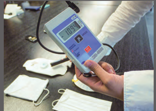
A reading on a static meter shows that an N95 mask has a negative voltage of minus 1,094 volts.
