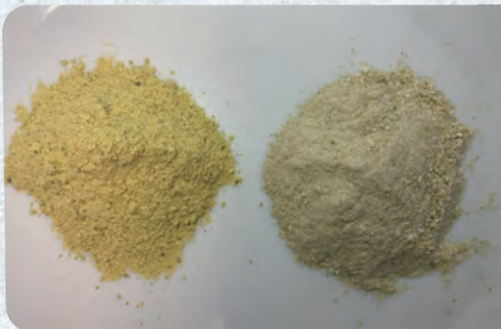
Making powder : Pulverized vegetable and fruit waste
