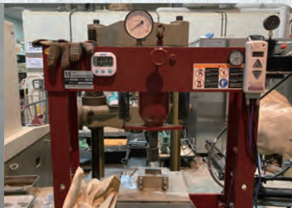
Molding : Heat-pressing machine
