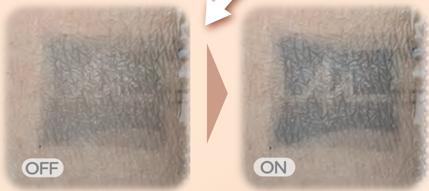
A display that adheres to skin wrinkles (under development). The color becomes darker when the power supply is turned on.
