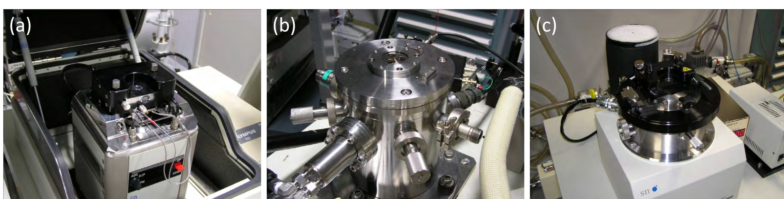
Multi-functional SPM equipments: (a) air type, (b)/(c) high vacuum and variable temperature type
