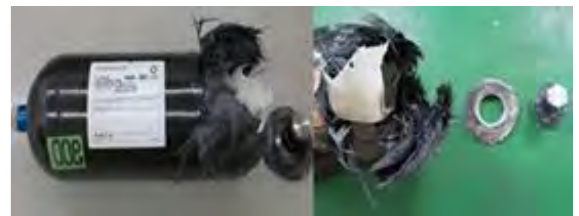
Validation of simulation by tank burst test
