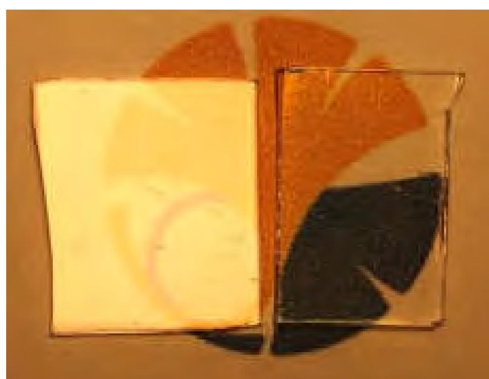
Reflection image of glass before (left) and after (right) surface treatment
