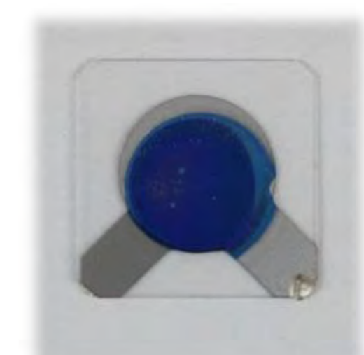
Analysis of the insertion/extraction behavior of Mg ions by electrochemical QCM
