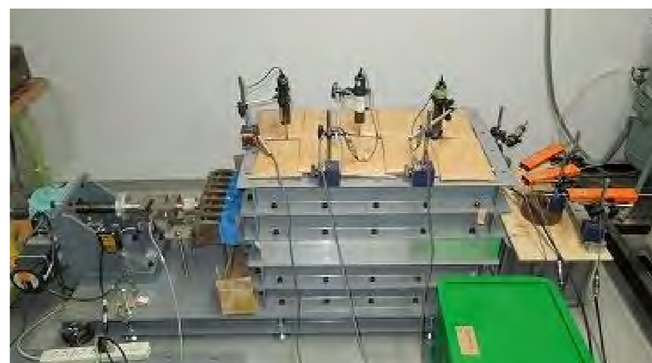
Pull-out test and shaking table model test on newly developed Geo-cell reinforced retaining wall
