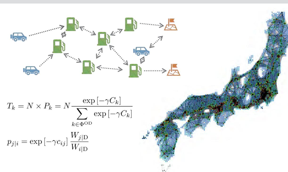
$$T_k = N \times P_k = N \frac{\exp[-\gamma C_k]}{\sum_{k \in \text{grid}} \exp[-\gamma C_k]}$$
