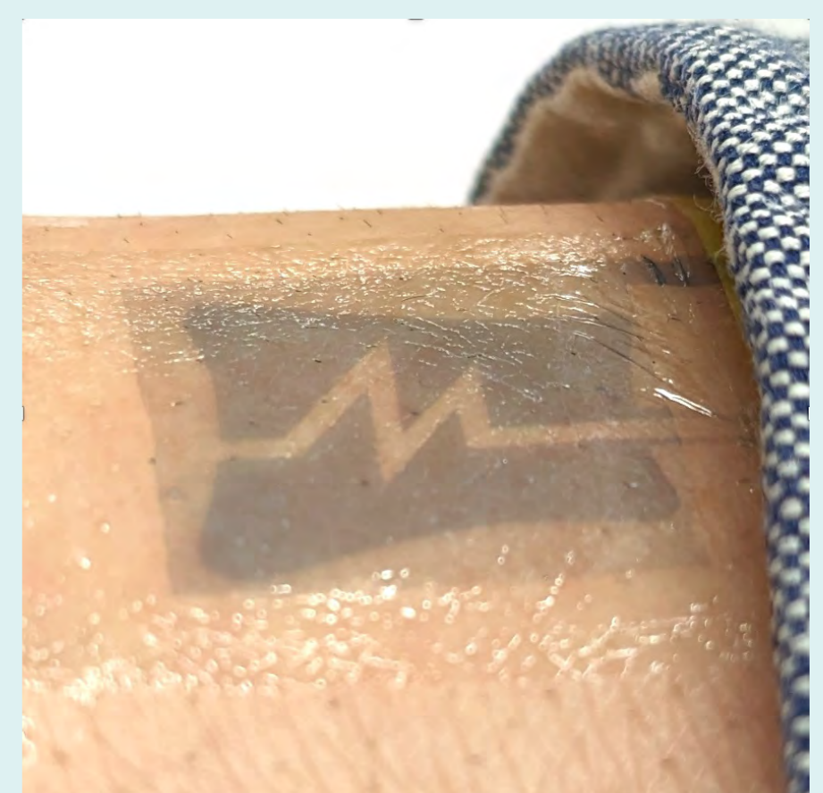
Exceptional skin-conformability of the soft and stretchable display
